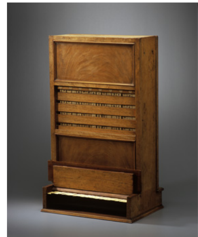
The logic piano: a mechanical computer designed by Jevons in 1866 to solve problems in logic. Inv. 18230. ©History of Science Museum, University of Oxford. Usage granted until 2031.
